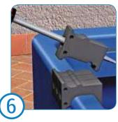
The electrical cables are passed through special patented rubber cable glands that ensure a perfectly airtight seal. Before fitting the cable, perforate the chosen cable glands with a sharp tool, but leave the others intact to keep liquids or smells inside the unit.
